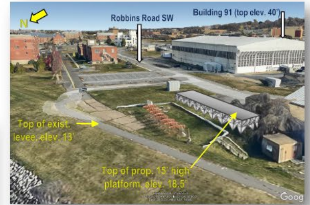
Looking South-East from Potomac River edge towards proposed 15' high Localizer Antenna platform at JBAB.
